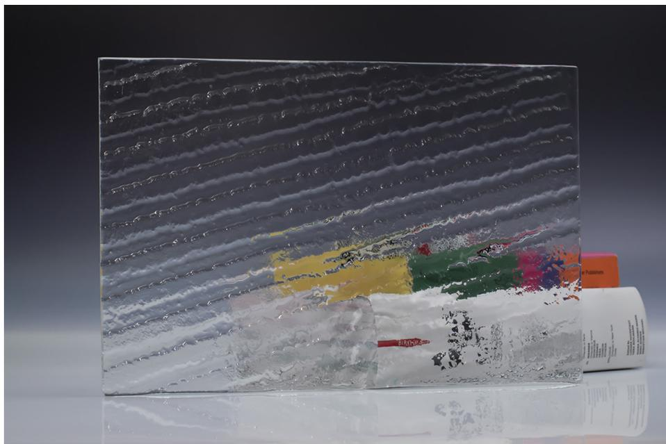
Texture glass is shaped in a kiln to reflect the imprinted shape of the mold it is placed on before heating. Our designers have created a collection inspired by nature, consisting of eight different textures that can be partially transparent, and if combined with a colored background or mirror, they can be more textured or glittery, and the colors even brighter. These designs allow for separation and privacy in many private and commercial applications.
